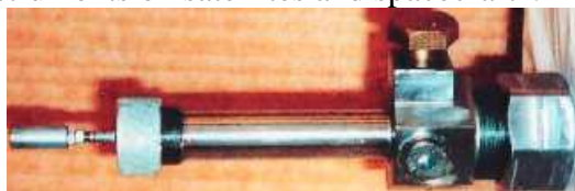
Fig. 4. Photo of self-contained actuator for space applications.
