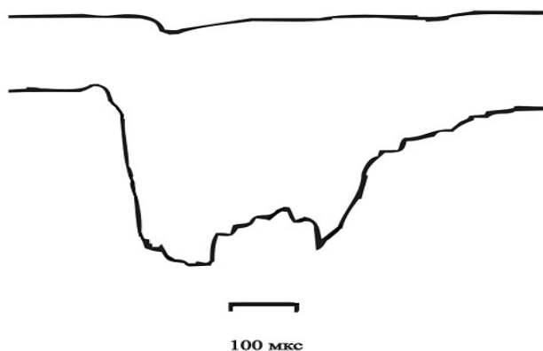
Figure 3. The oscillograms, fixing process of deformation of the tubular shock-tube: 1 - when
